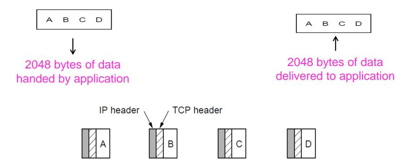
TCP default data or payload size is 536 bytes. 4 TCP segments, each with 536 bytes of data in first 3 segments and 440 bytes data in the 4<sup>th</sup> segment carried in 4 IP packets
