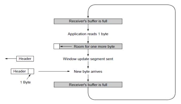
Receiver application reads single bytes, so sender always sends one byte segments
