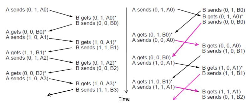
Notation is (seq, ack, frame number). Asterisk indicates frame accepted by network layer .
