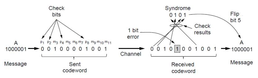
(11, 7) Hamming code adds 4 check bits and can correct 1 error
