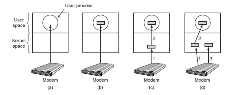
(a) Unbuffered input. (b) Buffering in user space. (c)
