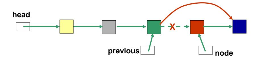
3. Make the node that previous points to, point to the node next to the one that to be deleted
