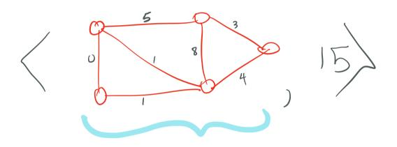
This is an example of a Graph with a weight function on its edges.
