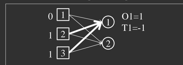
Slightly reduce weights on inputs with 1 Slightly Increase weight on input with 0
