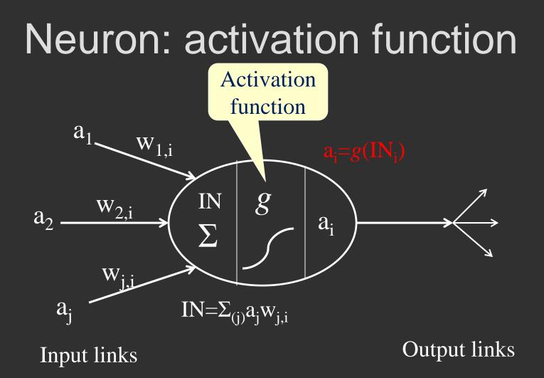
Activation function should be threshold function
