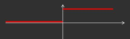
Example of threshold function: y(x)=0 if x<0y(x)=1 if  $(x\geq 0)$  (neuron fires)
