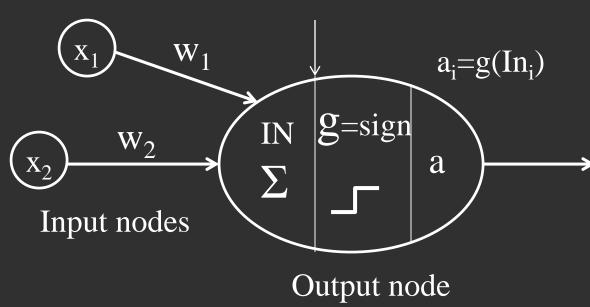
Objective of Perceptron learning: determine the optimal values of weights to separate all labeled instances by a hyperplane The output node gets activated only if  $\Sigma x_i w_i + t > 0$
